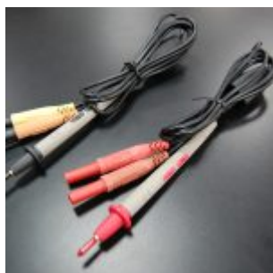
4-Wire Test Leads (M3500-opt08).
