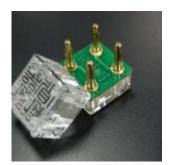
The M3500-OPT12 supports the multi-function measurements, including 2-/4wired Ohm, Voltage, Freq., Period, Thermocouple, RTD, and indirect Current (Shunt via Software's MX+B).
