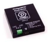
The 3853 Enclosure is designed to protect the 1024 – PhidgetRFID Read/Write while still giving you access to the USB port and terminal block through openings in the enclosure. Tags can be read by placing them flat on the face of the enclosure where the Phidgets logo is.
