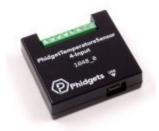
The 3855 Enclosure is designed to protect the 1048 — PhidgetTemperatureSensor 4-Input while still giving you access to the USB port through an opening in the enclosure.
