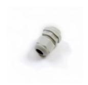
When you need to pass a cable into a waterproof enclosure you need to drill a hole in the enclosure. This of course makes it no longer water tight. To solve this, you can use a cable gland to make a water tight seal around the cable you are passing into the enclosure. This gland is suitable for cables from  $3.5-8 \,\mathrm{mm}$  in diameter.
