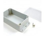
With an IP65 rating, this enclosure will protect your Phidgets from the elements. With proper installation of the foam rubber sealing ring, even the heaviest of rainstorms won't get through. All that is needed to assemble is a Phillips screwdriver. The clear lid allows quick visual inspection of the equipment inside without having to disassemble the box.
