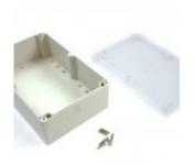
With an IP65 rating, this enclosure will protect your Phidgets from the elements. With proper installation of the foam rubber sealing ring, even the heaviest of rainstorms won't get through. All that is needed to assemble is a Phillips screwdriver. The clear lid allows quick visual inspection of the equipment inside without having to disassemble the box.
