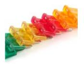
You can use these fuses to protect your system if you have high current power supplies or batteries. When semiconductors fail, they often become a short circuit, and will glow white-hot if the power supply is powerful enough. A properly sized fuse can interrupt the flow, preventing possible fire or damage to other components in the system.
