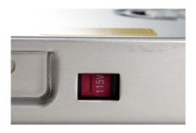
Caution: Before using this power supply, ensure that you flip the red switch on the side of the supply so it displays the voltage that matches your country's mains voltage.
