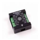
Note: The 1046\_0B is identical to the 1046\_0, except that it comes preassembled in a plastic shell enclosure and you have the option of which length of USB cable you want to include.
