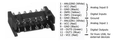
Wires 1,2,3 and wires 7,8,9 end with a female connector designed to take the Phidget sensor cable. The other wires are loose.
