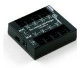
Light up your world with this 32-output dimmable LED controller. Precise control of your LEDs has never been easier, and it only takes one VINT port on your hub. The LED1000 connects to a port on a **VINT Hub**. See the "Comaptible Products" tab for a list of hubs.
