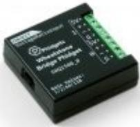
Bridge-based sensors are a common type of resistive sensor that produce a very small voltage drop. Load cells, strain gauges, pressure sensors, and piezoelectric sensors are all examples of sensors that usually operate in this way. In order to measure these tiny voltage changes, you need a Wheatstone bridge input. The Wheatstone Bridge Phidget uses a high-resolution ADC to read up to two of these signals and plugs into any **VINT port**. See the “Compatible Products” tab for a list of VINT Hubs.
