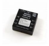
The Wireless VINT Hub is the easiest way to use Phidgets in locations far away from a computer. As long as there's a local WiFi signal and a nearby power outlet, this hub will make any attached Phidgets accessible to computers on the network without having to worry about using long cables. You can also wire it directly into your modem or network switch using an ethernet cable.
