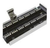
Provides convenient screw terminals for the DB37 connector on the LabJack U6, UE9, and T7. Includes a screwdriver. Is compatible with LJTick signal-conditioning modules.
