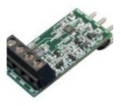
Provides a pair of 14-bit analog outputs with a range of +/- 10 volts. Plugs into any digital I/O block, and thus up to 10 of these can be used per LabJack to add 20 analog outputs. Works with the T7 and any UD family device (U3/U6/UE9), except for U3 hardware revision 1.20 (U3A)
