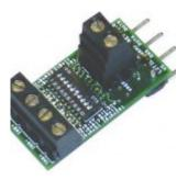
Signal-conditioning module provides two instrumentation amplifiers ideal for low-level signals such as bridge circuits (e.g. strain gauges) and thermocouples. Each amplifier converts a differential input to single-ended. The LJTIA has switches to choose from 5 gain settings (x1, x11, x51, x201, or custom) and two output voltage offsets. The 4-pin design plugs into the standard AIN/AIN/GND/VS screw terminal block found on newer LabJacks such as the U3, U6, UE9, and T7.
