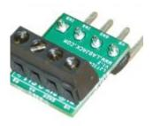
The LJTick-RelayDriver (LJTRD) allows 2 digital I/O lines on a U3, U6, UE9, or T7 to each control a relay or other moderate load. The 4-pin design plugs into the standard DIO/DIO/GND/VS screw terminal block found on newer LabJacks such as the U3, U6, UE9, and T7. Each DIO controls a switch to ground (i.e. open-collector) that can hold off up to 50 volts and can sink up to 200 mA.
