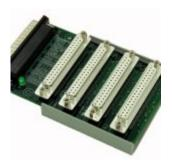
The Mux80 is an analog input expansion board that increases the number of analog inputs possible for a LabJack unit. It can be connected to a U6, UE9, or T7 directly through the DB37 connector. Ten of the LabJack's analog inputs are multiplexed (1:8 each) by the Mux80, and 4 are left untouched on AIN0-3 screw terminals, bringing the total number of available analog inputs to 84.
