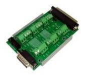
The PS12DC is a power switching board designed for medium to low current DC power switching applications. Controlled through 12 digital outputs, the board can switch power sources ranging from 5 to 28V DC. Attach the PS12DC to the DB15 connector presented on all compatible devices, and toggle the states of the EIO and CIO digital output lines to turn the switches on/off.
