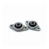
Bearings provide mechanical support for rotating shafts while not interfering with the rotation significantly. This bearing is a flange bearing meaning that it mounts to a surface that is perpendicular to the shaft being supported.
