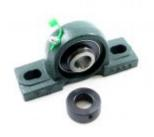
Bearings provide mechanical support for rotating shafts while not interfering with the rotation significantly. This bearing is a pillow block bearing meaning that it mounts to a surface that is parallel to the shaft being supported.
