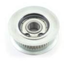
Idler pulleys are standard pulleys with an integrated bearing. This allows them to spin freely without impeding the rotation in your system. This is useful for when you want an adjustable way to tension a belt system that doesn't impact the movement of the belt or place additional load on the motor.
