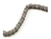
0.25" Pitch roller chain, for use with #25 sprockets. Roller chain can handle more load than belt systems, and is normally used for rotary systems. Chain can be used to create linear motion, but has to be run with a bit of slack in the system. Sold by the meter.
