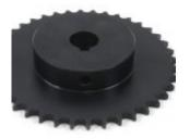
Hardened steel sprocket for half inch (1/2") roller chain. There is a 25mm bore with keyway, set screws and key.
