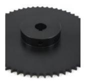
Hardened steel sprocket for half inch (1/2") roller chain. There is a 25mm bore with keyway, set screws and key.
