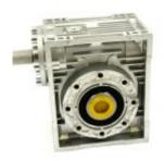
Worm drives are compact gearboxes with high output torque for their size. This particular gearbox is rated for 163Nm and is compatible with 63 Series 25mm output shafts. The input shaft is 19mm and you will couple to a rotating power source — typically through a jaw coupling, timing belt pulley or chain sprocket.
