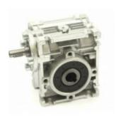
Worm drives are compact gearboxes with high output torque for their size. This particular gearbox is rated for 20Nm and is compatible with 30 Series 14mm output shafts. The input shaft is 9mm and you will couple to a rotating power source — typically through a jaw coupling, timing belt pulley or chain sprocket.
