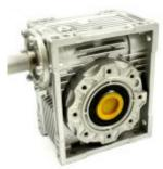
Worm drives are compact gearboxes with high output torque for their size. This particular gearbox is rated for 234Nm and is compatible with 75 Series 35mm output shafts. The input shaft is 24mm and you will couple to a rotating power source — typically through a jaw coupling, timing belt pulley or chain sprocket.
