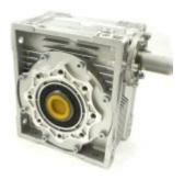
Worm drives are compact gearboxes with high output torque for their size. This particular gearbox is rated for 418Nm and is compatible with 90 Series 35mm output shafts. The input shaft is 24mm and you will couple to a rotating power source — typically through a jaw coupling, timing belt pulley or chain sprocket.
