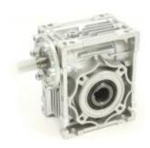
Worm drives are compact gearboxes with high output torque for their size. This particular gearbox is rated for 45Nm and is compatible with 40 Series 19mm output shafts. The input shaft is 11mm and you will couple to a rotating power source — typically through a jaw coupling, timing belt pulley or chain sprocket.
