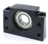
Both ends of a ball screw need to be supported by a bearing. This bearing is used on the free end of the screw. The snap ring that is included is used to secure the bearing in place on the screw. This bearing is for 25mm ball screws.
