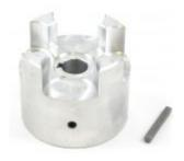
This jaw type half-coupling can be used to connect a 0.5" shaft to another shaft. It is held in place by two set screws, and fits together with another series 24 jaw coupling of any shaft size with a hard elastomer spider in between. See the "Compatible Products" tab for a complete list of compatible couplings and spiders.
