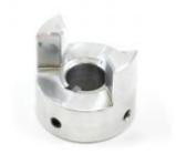
This jaw type half-coupling can be used to connect a 10mm shaft to another shaft. It is held in place by two set screws, and fits together with another series 12 jaw coupling of any shaft size with a hard elastomer spider in between. See the "Compatible Products" tab for a complete list of compatible couplings and spiders.
