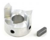
This jaw type half-coupling can be used to connect a 11mm shaft to another shaft. It is held in place by two set screws, and fits together with another series 12 jaw coupling of any shaft size with a hard elastomer spider in between. See the "Compatible Products" tab for a complete list of compatible couplings and spiders.
