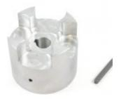
This jaw type half-coupling can be used to connect a 17mm shaft to another shaft. It is held in place by two set screws, and fits together with another series 38 jaw coupling of any shaft size with a hard elastomer spider in between. See the "Compatible Products" tab for a complete list of compatible couplings and spiders.
