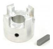
This jaw type half-coupling can be used to connect a 24mm shaft to another shaft. It is held in place by two set screws, and fits together with another series 24 jaw coupling of any shaft size with a hard elastomer spider in between. See the "Compatible Products" tab for a complete list of compatible couplings and spiders.
