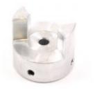
This jaw type half-coupling can be used to connect a 4mm shaft to another shaft. It is held in place by two set screws, and fits together with another series 12 jaw coupling of any shaft size with a hard elastomer spider in between. See the "Compatible Products" tab for a complete list of compatible couplings and spiders.
