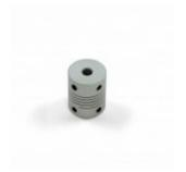
This beam type coupling can be used to connect two 5mm shafts together. Each shaft is held in place by two set screws, allowing for easy installation. The spiral cut design allows for up to 2?° of bending from angular misalignment and up to 0.12mm eccentric misalignment.
