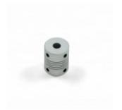
This beam type coupling can be used to connect two 6mm shafts together. Each shaft is held in place by two set screws, allowing for easy installation. The spiral cut design allows for up to 2B° of bending from angular misalignment and up to 0.12mm eccentric misalignment.
