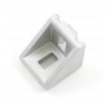
This bracket strengthens 90?° joints in your system. It is suitable for use with PG30 extrusions. You will need 2 M6x14 bolts with washers and nuts to install. We recommend this part as a reinforcing component rather than the sole means for connecting 2 profiles together.
