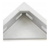
This bracket strengthens 90?° joints in your system. These brackets are larger and sturdier than the TSL4103 variant so will give even more rigidity to your structure. It is suitable for use with PG30 extrusions. You will need 4 M6x14 bolts with washers and nuts to install. We recommend this part as a reinforcing component rather than the sole means for connecting 2 profiles together.
