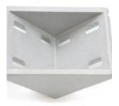
This bracket strengthens 90?° joints in your system. It is suitable for use with the double-wide PG30 extrusions. You will need 8 M6x14 bolts with washers and nuts to install. We recommend this part as a reinforcing component rather than the sole means for connecting 2 profiles together.
