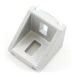
This bracket strengthens 90?° joints in your system. It is suitable for use with PG40 extrusions. You will need 2 M8x20 bolts with washers and nuts to install. We recommend this part as a reinforcing component rather than the sole means for connecting 2 profiles together.
