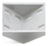
This bracket strengthens 90?° joints in your system. It is suitable for use with the double-wide PG40 extrusions. You will need 8 M8x20 bolts with washers and nuts to install. We recommend this part as a reinforcing component rather than the sole means for connecting 2 profiles together.
