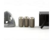
This bracket is used to connect 3 extrusion pieces into a 3d corner such as the vertex of a cube. You are required to use an M12 tap to bore out the end of the extrusions into which you insert the included bore reducer. Then just bolt the bracket on with an M6x20 bolt. Ideally you want to use a bolt with the DIN 7991 head style but it doesn't actually matter too much.
