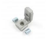
This bracket allows you to connect extrusions at right angles to one another. It is suitable for use with PG30 extrusions. They are not as strong as the screw or butt connectors but are fast and easy to use. A 3mm hex drive is required to tighten the set screw.
