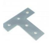
This bracket is a steel plate to add extra stiffness to T joints. You need 5 sets of M8x12 bolts with nuts and washers. Compatible with PG40 extrusions.
