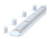
This bar is used to join 2 extrusions together in a straight line fashion. A 2.5mm hex drive is required to tighten the set screws. You should use 2 bars per joint though you can use as many as 4 if extra strength is desired. For use with PG30 extrusions.
