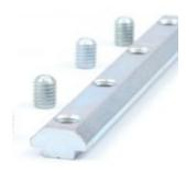
This bar is used to join 2 extrusions together in a straight line fashion. A 2.5mm hex drive is required to tighten the set screws. You should use 2 bars per joint though you can use as many as 4 if extra strength is desired. For use with PG40 extrusions.
